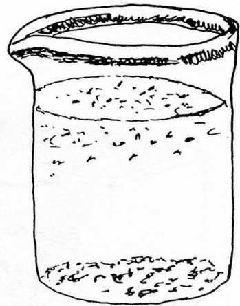
FIGURE 5-13. The beaker method for heavy liquid separation.
